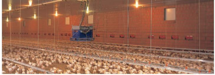
Heat can be supplied to broilers by a hot-water heater – Big Dutchman's HeatMaster
