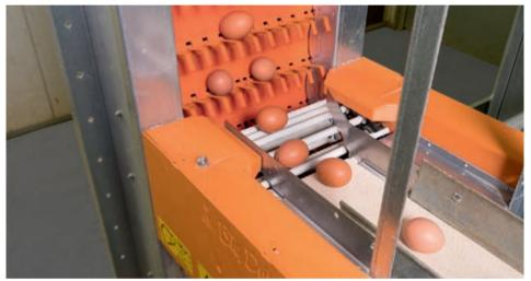
Egg transfer from the longitudinal belt to the rod conveyor and onto the elevator chain
