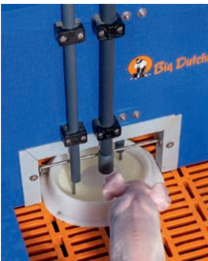
A sensor checks the feed level in the trough and informs the 510 pro computer
