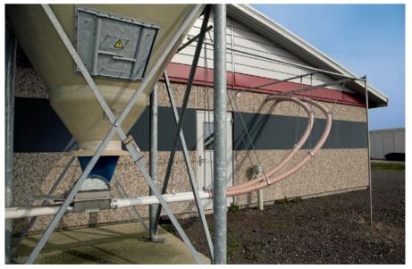
Use of FlexVey PUR in combination with a rigid FlexVey tube
