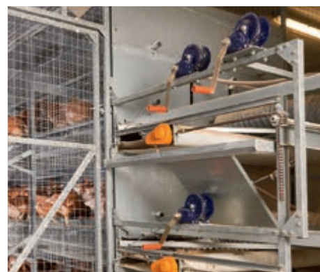
A manual winch in each tier opens the sliding fronts simultaneously and easily
