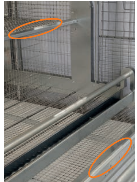
View into a compartment: sheet metal perches in both tiers ensure a secure foothold
