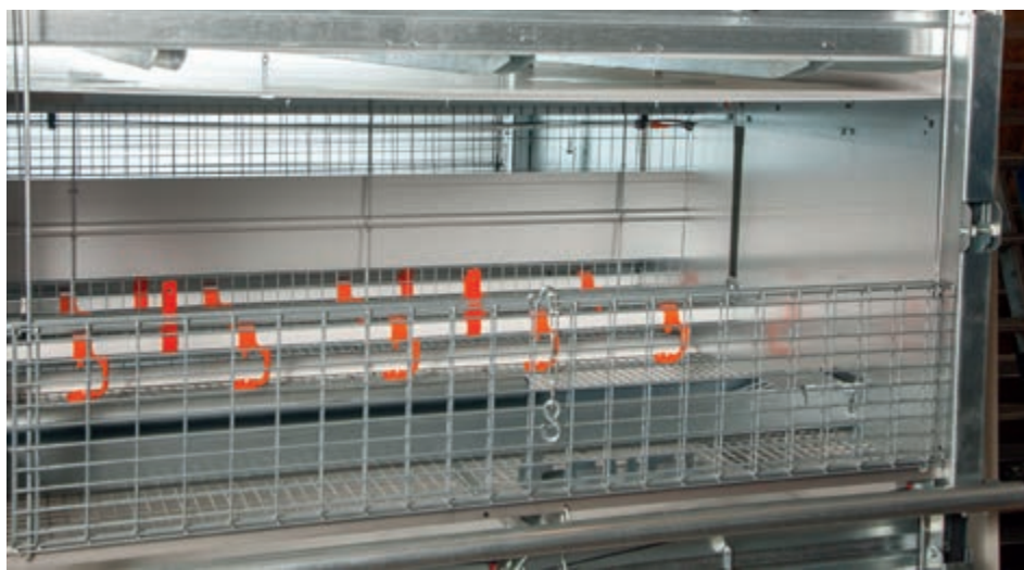
A heating pipe in the bottom tier supplies direct heat during the first days
