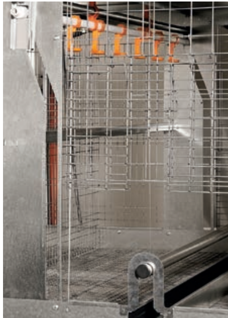
Open partition, height-adjustable perch above the trough, height-adjustable drinker line
