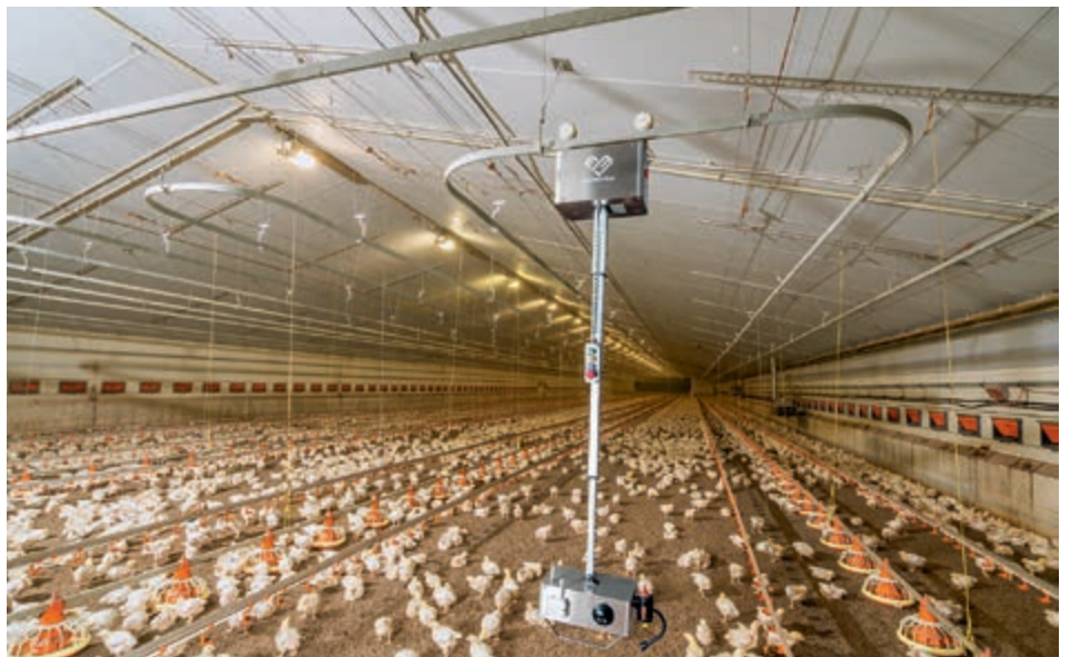
The height of ChickenBoy can be adjusted by a telescopic arm
