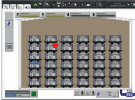
Light and water control in a layer system, display of the currently active rinsing process
