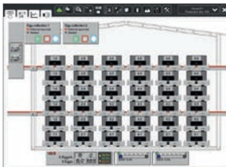
Egg counters per longitudinal egg belt register every egg
