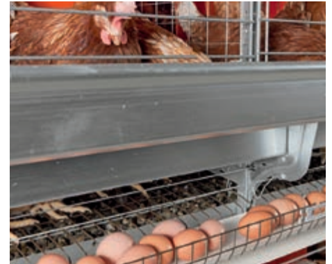
EggSaver in raised position → the eggs can roll onto the longitudinal egg belt
