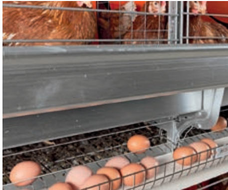
EggSaver in lowered position → the eggs are slowed down carefully
