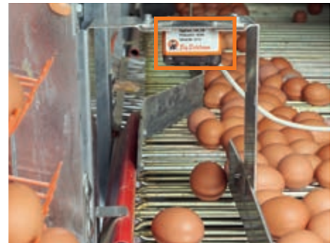
EggCam 140 at the egg cross belt, covering a width of up to 14 cm
