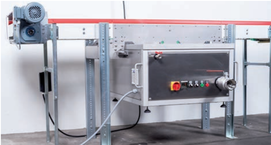
Compact cleaning unit – requires little space and no deflection unit above the conveyor
