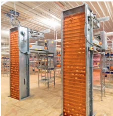
EC elevator in a multi-level house
